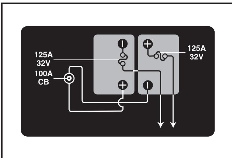
Figure 11. Battery Configuration
