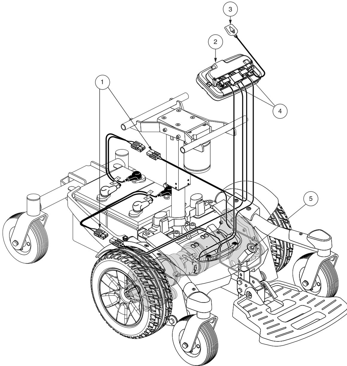
Figure 6. Jazzy Select 6 with Power Seat Electrical Components
