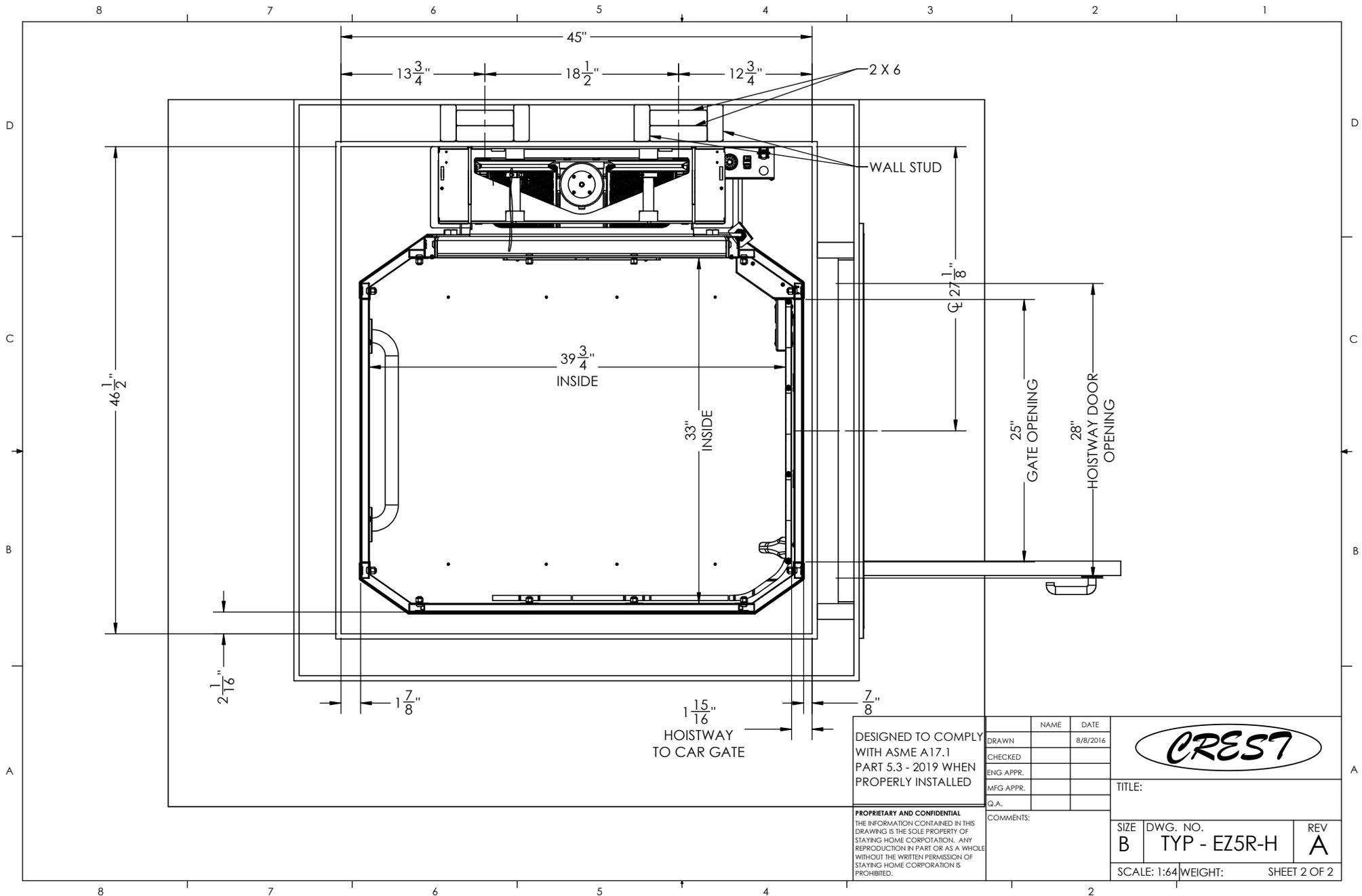
DESIGNED TO COMPLY WITH ASME A17.1 PART 5.3 - 2019 WHEN PROPERLY INSTALLED
