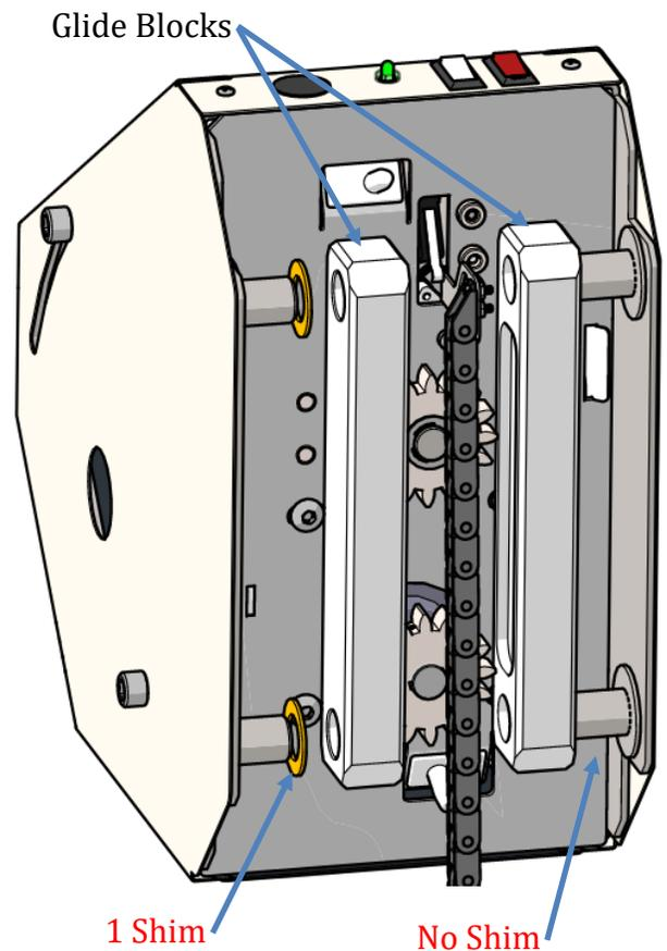
Flip the red RESET/OFF switch to the RESET position. The lift will beep and is now ready to be run down onto the gear rack using the black INSTALLATION SWITCH on top of the chassis.
