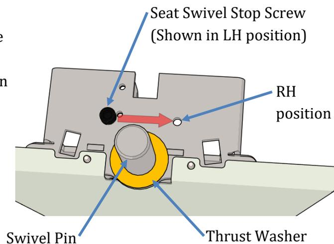
Place the seat assembly onto the swivel pin. It may be necessary to lubricate the swivel pin.
