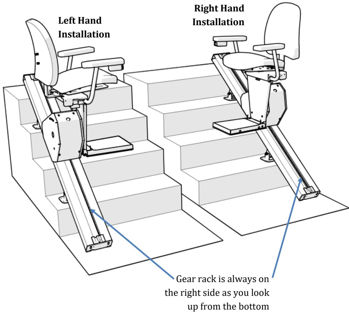
Apply a light coat of lithium grease on the gear rack and vertical sides of the track .
