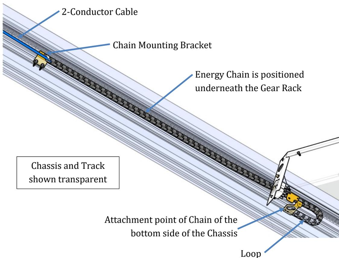
Adjust position of travel cable so there is a small loop in the Chain.
