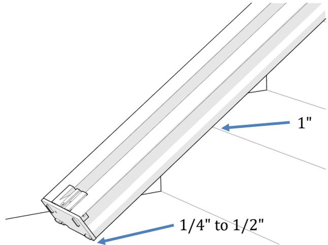
Install rail brackets by loosening the screws and snapping each bracket edge into the slot or slide the brackets on from the top of the rail. The rail brackets are designed to lean the track toward the wall to offset the weight of the unit and user, therefore, the nuts on brackets should be on the staircase side (toward the middle of the staircase).
