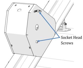
Remove the front cover from the footrest assembly (two phillips head screws).
