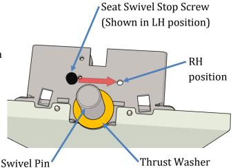
Place the seat assembly onto the swivel pin. It may be necessary to lubricate the swivel pin.
